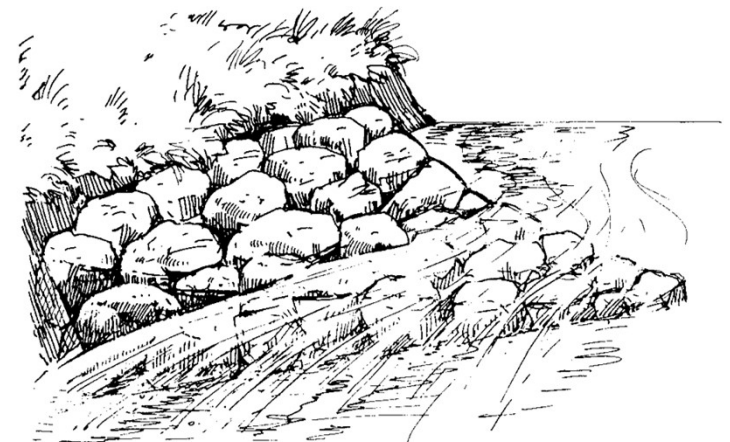
Bank spur made of hydraulic stones
