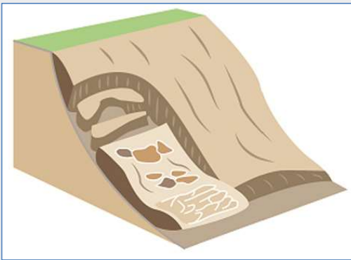
b) Translational slides occurs when the failure surface is approximately flat or slightly undulated
